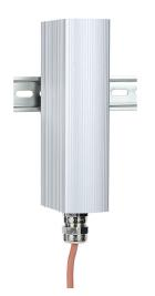
Stego enclosure heater, hazardous location rated, 100W heating capacity, high performance cartridge heating element, 230 VAC operating voltage, 35mm DIN rail mount.
