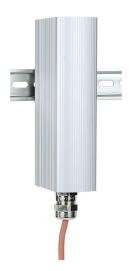
Stego enclosure heater, hazardous location rated, 100W heating capacity, high performance cartridge heating element, 230 VAC operating voltage, 35mm DIN rail mount.
