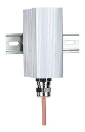
Stego enclosure heater, hazardous location rated, 50W heating capacity, high performance cartridge heating element, 120 VAC operating voltage, 35mm DIN rail mount.
