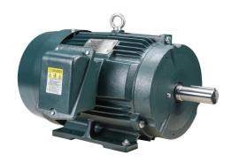
Toshiba SD premium efficiency AC induction motor, high-performance inverter duty and severe duty, 20hp, 3-phase, 230/460 VAC, 3600rpm, TEFC, NEMA 256T frame, cast iron, rigid base mount.
