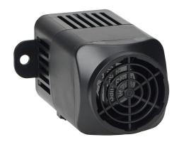
Stego StegoJet series compact directional cooling fan, for precise cooling of heat sources inside an enclosure, 100-240 VAC operating voltage, 50/60 Hz, panel mount, IP20.
