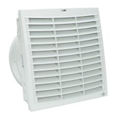
Stego Filter Fan Plus FPO exhaust fan, side mount, 256 CFM, 115 VAC operating voltage, G3 (coarse) filter mat, NEMA 12, indoor use only, 11.46 x 11.46in enclosure cutout, RAL 7035 light gray.
