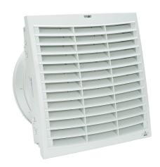
Stego Filter Fan Plus FPO exhaust fan, side mount, 414 CFM, 115 VAC operating voltage, with air flaps, NEMA 12, indoor use only, 11.46 x 11.46in enclosure cutout, RAL 7035 light gray.
