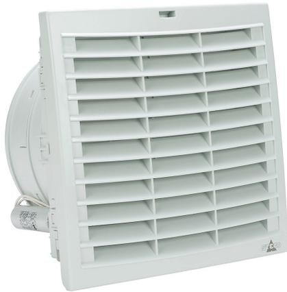
Stego Filter Fan Plus FPO exhaust fan, side mount, 342 CFM, 115 VAC operating voltage, with air flaps, NEMA 12, indoor use only, 8.78 x 8.78in enclosure cutout, RAL 7035 light gray.
