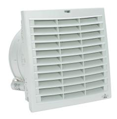
Stego Filter Fan Plus FPO exhaust fan, side mount, 342 CFM, 115 VAC operating voltage, with air flaps, NEMA 12, indoor use only,  $8.78 \times 8.78$  in enclosure cutout, RAL 7035 light gray.
