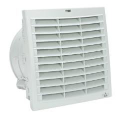
Stego Filter Fan Plus FPO exhaust fan, side mount, 316 CFM, 230 VAC operating voltage, with air flaps, NEMA 12, indoor use only,  $8.78 \times 8.78$  in enclosure cutout, RAL 7035 light gray.
