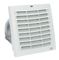
Stego Filter Fan Plus FPO exhaust fan, side mount, 184 CFM, 115 VAC operating voltage, with air flaps, NEMA 12, indoor use only,  $6.93 \times 6.93$  in enclosure cutout, RAL 7035 light gray.
