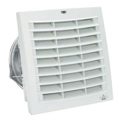
Stego Filter Fan Plus FPO exhaust fan, side mount, 106 CFM, 230 VAC operating voltage, G3 (coarse) filter mat, NEMA 12, indoor use only, 6.93 x 6.93in enclosure cutout, RAL 7035 light gray.
