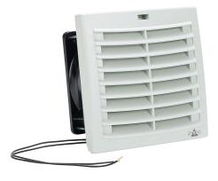
Stego Filter Fan Plus FPO exhaust fan, side mount, 39 CFM, 115 VAC operating voltage, G3 (coarse) filter mat, NEMA 12, indoor use only, 4.88 x 4.88in enclosure cutout, RAL 7035 light gray.
