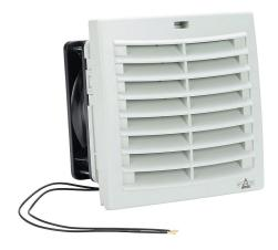
Stego Filter Fan Plus FPO exhaust fan, side mount, 69 CFM, 115 VAC operating voltage, with air flaps, NEMA 12, indoor use only, 4.88 x 4.88in enclosure cutout, RAL 7035 light gray.
