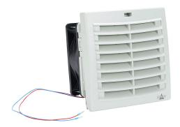
Stego Filter Fan Plus FPO exhaust fan, side mount, 70 CFM, 12 VDC operating voltage, with air flaps, NEMA 12, indoor use only, 4.88 x 4.88in enclosure cutout, RAL 7035 light gray.
