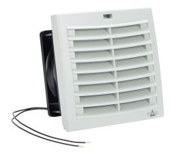
Stego Filter Fan Plus FPO exhaust fan, side mount, 32 CFM, 230 VAC operating voltage, G3 (coarse) filter mat, NEMA 12, indoor use only, 4.88 x 4.88in enclosure cutout, RAL 7035 light gray.
