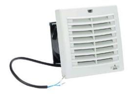
Stego Filter Fan Plus FPO exhaust fan, side mount, 14 CFM, 115 VAC operating voltage, G3 (coarse) filter mat, NEMA 12, indoor use only,  $3.62 \times 3.62$  in cutout, RAL 7035 light gray.
