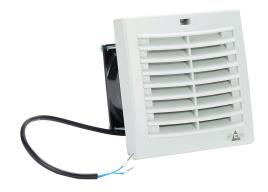
Stego Filter Fan Plus FPO exhaust fan, side mount, 14 CFM, 115 VAC operating voltage, G3 (coarse) filter mat, NEMA 12, indoor use only, 3.62 x 3.62in enclosure cutout, RAL 7035 light gray.
