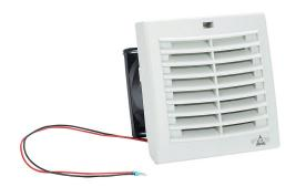
Stego Filter Fan Plus FPO exhaust fan, side mount, 19 CFM, 48 VDC operating voltage, with air flaps, NEMA 12, indoor use only,  $3.62 \times 3.62$  in enclosure cutout, RAL 7035 light gray.
