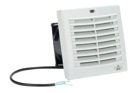
Stego Filter Fan Plus FPO exhaust fan, side mount, 11 CFM, 230 VAC operating voltage, G3 (coarse) filter mat, NEMA 12, indoor use only, 3.62 x 3.62in enclosure cutout, RAL 7035 light gray.
