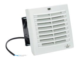
Stego Filter Fan Plus FPO exhaust fan, side mount, 14 CFM, 230 VAC operating voltage, with air flaps, NEMA 12, indoor use only,  $3.62 \times 3.62$  in enclosure cutout, RAL 7035 light gray.
