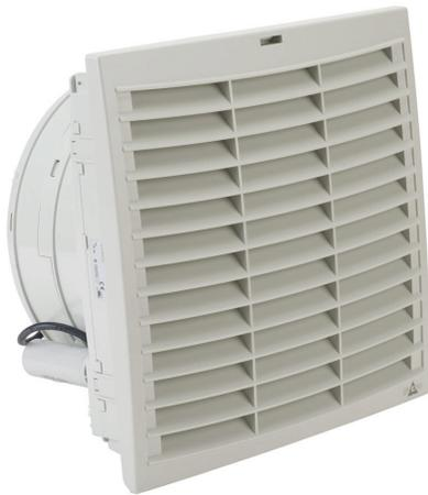
Stego Filter Fan Plus FPI intake fan, side mount, 391 CFM, 115 VAC operating voltage, G3 (coarse) filter mat, NEMA 12, indoor use only, 11.46 x 11.46in enclosure cutout, RAL 7035 light gray.
