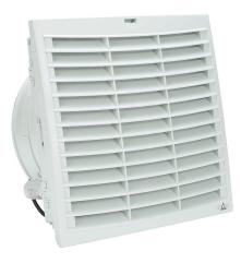
Stego Filter Fan Plus FPI intake fan, side mount, 232 CFM, 115 VAC operating voltage, G3 (coarse) filter mat, NEMA 12, indoor use only, 11.46 x 11.46in enclosure cutout, RAL 7035 light gray.
