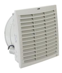
Stego Filter Fan Plus FPI intake fan, side mount, 367 CFM, 230 VAC operating voltage, G3 (coarse) filter mat, NEMA 12, indoor use only, 11.46 x 11.46in enclosure cutout, RAL 7035 light gray.
