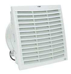
Stego Filter Fan Plus FPI intake fan, side mount, 255 CFM, 230 VAC operating voltage, G3 (coarse) filter mat, NEMA 12, indoor use only, 11.46 x 11.46in enclosure cutout, RAL 7035 light gray.
