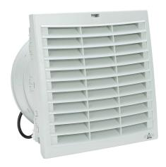
Stego Filter Fan Plus FPI intake fan, side mount, 180 CFM, 230 VAC operating voltage, G3 (coarse) filter mat, NEMA 12, indoor use only, 8.78 x 8.78in enclosure cutout, RAL 7035 light gray.
