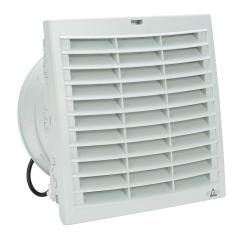
Stego Filter Fan Plus FPI intake fan, side mount, 180 CFM, 230 VAC operating voltage, G3 (coarse) filter mat, NEMA 12, indoor use only,  $8.78 \times 8.78$  in enclosure cutout, RAL 7035 light gray.
