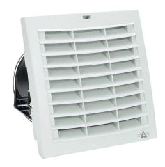
Stego Filter Fan Plus FPI intake fan, side mount, 106 CFM, 12 VDC operating voltage, G3 (coarse) filter mat, NEMA 12, indoor use only,  $6.93 \times 6.93$  in enclosure cutout, RAL 7035 light gray.
