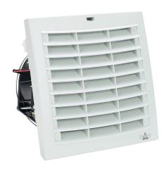
Stego Filter Fan Plus FPI intake fan, side mount, 105 CFM, 24 VDC operating voltage, G3 (coarse) filter mat, NEMA 12, indoor use only,  $6.93 \times 6.93$  in enclosure cutout, RAL 7035 light gray.
