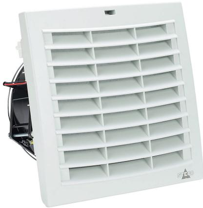
Stego Filter Fan Plus FPI intake fan, side mount, 105 CFM, 24 VDC operating voltage, G3 (coarse) filter mat, NEMA 12, indoor use only, 6.93 x 6.93in enclosure cutout, RAL 7035 light gray.
