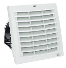
Stego Filter Fan Plus FPl intake fan, side mount, 100 CFM, 48 VDC operating voltage, G3 (coarse) filter mat, NEMA 12, indoor use only, 6.93 x 6.93in enclosure cutout, RAL 7035 light gray.
