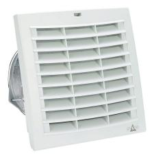
Stego Filter Fan Plus FPI intake fan, side mount, 100 CFM, 230 VAC operating voltage, G3 (coarse) filter mat, NEMA 12, indoor use only, 6.93 x 6.93in enclosure cutout, RAL 7035 light gray.
