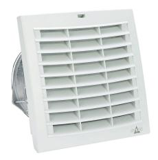
Stego Filter Fan Plus FPI intake fan, side mount, 100 CFM, 230 VAC operating voltage, G3 (coarse) filter mat, NEMA 12, indoor use only, 6.93 x 6.93in enclosure cutout, RAL 7035 light gray.
