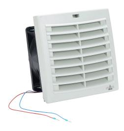
Stego Filter Fan Plus FPI intake fan, side mount, 45 CFM, 12 VDC operating voltage, G3 (coarse) filter mat, NEMA 12, indoor use only, 4.88 x 4.88in enclosure cutout, RAL 7035 light gray.
