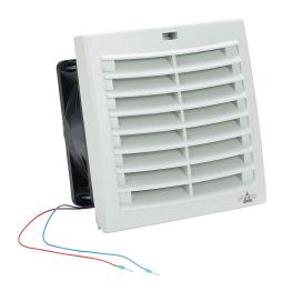
Stego Filter Fan Plus FPI intake fan, side mount, 45 CFM, 12 VDC operating voltage, G3 (coarse) filter mat, NEMA 12, indoor use only,  $4.88 \times 4.88$ in enclosure cutout, RAL 7035 light gray.
