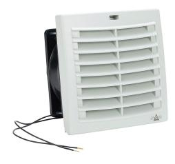
Stego Filter Fan Plus FPI intake fan, side mount, 31 CFM, 230 VAC operating voltage, G3 (coarse) filter mat, NEMA 12, indoor use only, 4.88 x 4.88in enclosure cutout, RAL 7035 light gray.
