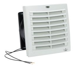
Stego Filter Fan Plus FPI intake fan, side mount, 31 CFM, 230 VAC operating voltage, G3 (coarse) filter mat, NEMA 12, indoor use only,  $4.88 \times 4.88$ in enclosure cutout, RAL 7035 light gray.
