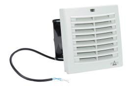
Stego Filter Fan Plus FPI intake fan, side mount, 14 CFM, 115 VAC operating voltage, G3 (coarse) filter mat, NEMA 12, indoor use only,  $3.62 \times 3.62$  in enclosure cutout, RAL 7035 light gray.
