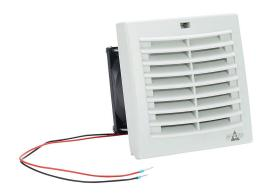
Stego Filter Fan Plus FPI intake fan, side mount, 13 CFM, 12 VDC operating voltage, G3 (coarse) filter mat, NEMA 12, indoor use only,  $3.62 \times 3.62$  in enclosure cutout, RAL 7035 light gray.
