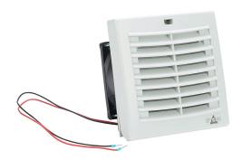
Stego Filter Fan Plus FPI intake fan, side mount, 13 CFM, 24 VDC operating voltage, G3 (coarse) filter mat, NEMA 12, indoor use only,  $3.62 \times 3.62$  in enclosure cutout, RAL 7035 light gray.
