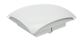
Stego exhaust fan, top mount, 203 CFM, 24 VDC operating voltage, G3 (coarse) filter mat, NEMA 3R, indoor use only, 9.69 x 9.69in enclosure cutout, RAL 7035 light gray.
