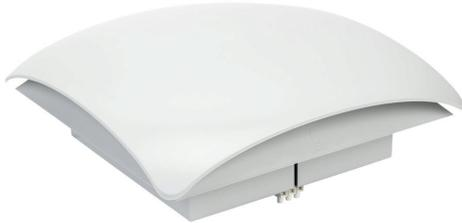
Stego exhaust fan, top mount, 203 CFM, 115 VAC operating voltage, G3 (coarse) filter mat, NEMA 3R, indoor use only, 9.69 x 9.69in enclosure cutout, RAL 7035 light gray.
