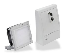
Stego Filter Fan intake fan, side mount, 12 CFM, 24 VDC operating voltage, M5 (medium) filter mat, NEMA 12, safe for outdoor use, 4.92 x 4.92in enclosure cutout, RAL 7035 light gray.
