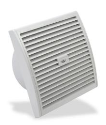
Stego Filter Fan intake fan, side mount, 372 CFM, 115 VAC operating voltage, G4 (coarse) filter mat, NEMA 12, indoor use only,  $9.84 \times 9.84$ in enclosure cutout, RAL 7035 light gray.
