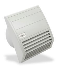
Stego Filter Fan intake fan, side mount, 136 CFM, 115 VAC operating voltage, G4 (coarse) filter mat, NEMA 12, indoor use only, 6.93 x 6.93in enclosure cutout, RAL 7035 light gray.
