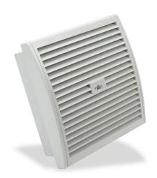
Stego Filter Fan intake fan, side mount, 176 CFM, 24 VDC operating voltage, G4 (coarse) filter mat, NEMA 12, indoor use only,  $9.84 \times 9.84$ in enclosure cutout, RAL 7035 light gray.
