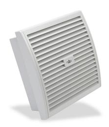
Stego Filter Fan intake fan, side mount, 202 CFM, 115 VAC operating voltage, G4 (coarse) filter mat, NEMA 12, indoor use only,  $9.84 \times 9.84$ in enclosure cutout, RAL 7035 light gray.
