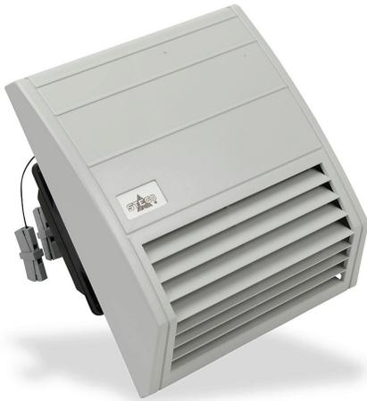
Stego Filter Fan intake fan, side mount, 60 CFM, 24 VDC operating voltage, G4 (coarse) filter mat, NEMA 12, indoor use only, 6.93 x 6.93in enclosure cutout, RAL 7035 light gray.
