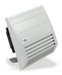
Stego Filter Fan intake fan, side mount, 69 CFM, 115 VAC operating voltage, G4 (coarse) filter mat, NEMA 12, indoor use only,  $6.93 \times 6.93$  in enclosure cutout, RAL 7035 light gray.
