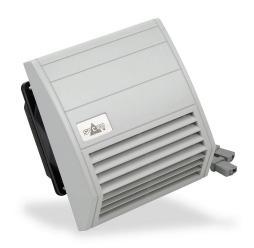
Stego Filter Fan intake fan, side mount, 32 CFM, 24 VDC operating voltage, G4 (coarse) filter mat, NEMA 12, indoor use only, 4.92 x 4.92in enclosure cutout, RAL 7035 light gray.
