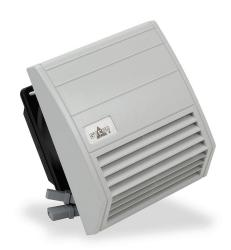
Stego Filter Fan intake fan, side mount, 37 CFM, 115 VAC operating voltage, G4 (coarse) filter mat, NEMA 12, indoor use only,  $4.92 \times 4.92$  in enclosure cutout, RAL 7035 light gray.
