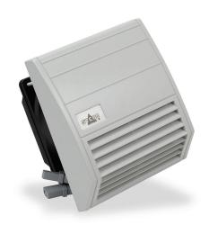
Stego Filter Fan intake fan, side mount, 37 CFM, 115 VAC operating voltage, G4 (coarse) filter mat, NEMA 12, indoor use only, 4.92 x 4.92in enclosure cutout, RAL 7035 light gray.
