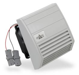
Stego Filter Fan intake fan, side mount, 12 CFM, 24 VDC operating voltage, G4 (coarse) filter mat, NEMA 12, indoor use only, 3.82 x 3.82in enclosure cutout, RAL 7035 light gray.
