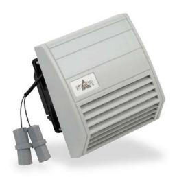
Stego Filter Fan intake fan, side mount, 14 CFM, 115 VAC operating voltage, G4 (coarse) filter mat, NEMA 12, indoor use only,  $3.82 \times 3.82$  in cutout, RAL 7035 light gray.
