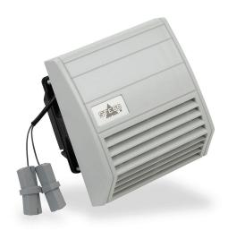
Stego Filter Fan intake fan, side mount, 14 CFM, 115 VAC operating voltage, G4 (coarse) filter mat, NEMA 12, indoor use only,  $3.82 \times 3.82$  in enclosure cutout, RAL 7035 light gray.
