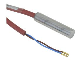
Stego enclosure heater, 9W heating capacity, PTC resistor heating element, 12-24 VAC/VDC operating voltage, panel mount.
