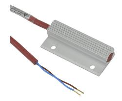
Stego enclosure heater, 13W heating capacity, PTC resistor heating element, 120-240 VAC/VDC operating voltage, panel mount.
