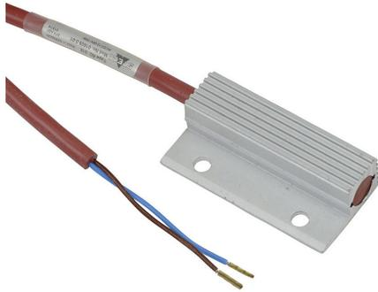
Stego enclosure heater, 10W heating capacity, PTC resistor heating element, 12-24 VAC/VDC operating voltage, panel mount.
