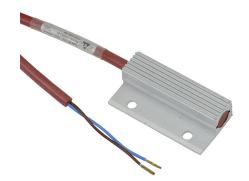
Stego enclosure heater, 10W heating capacity, PTC resistor heating element, 12-24 VAC/VDC operating voltage, panel mount.
