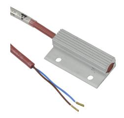
Stego enclosure heater, 10W heating capacity, PTC resistor heating element, 120-240 VAC/VDC operating voltage, panel mount.
