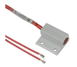
Stego enclosure heater, 8W heating capacity, PTC resistor heating element, 12-24 VAC/VDC operating voltage, panel mount.
